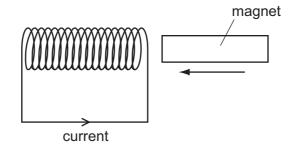
The magnet is then pulled out quickly from the same end of the coil.
